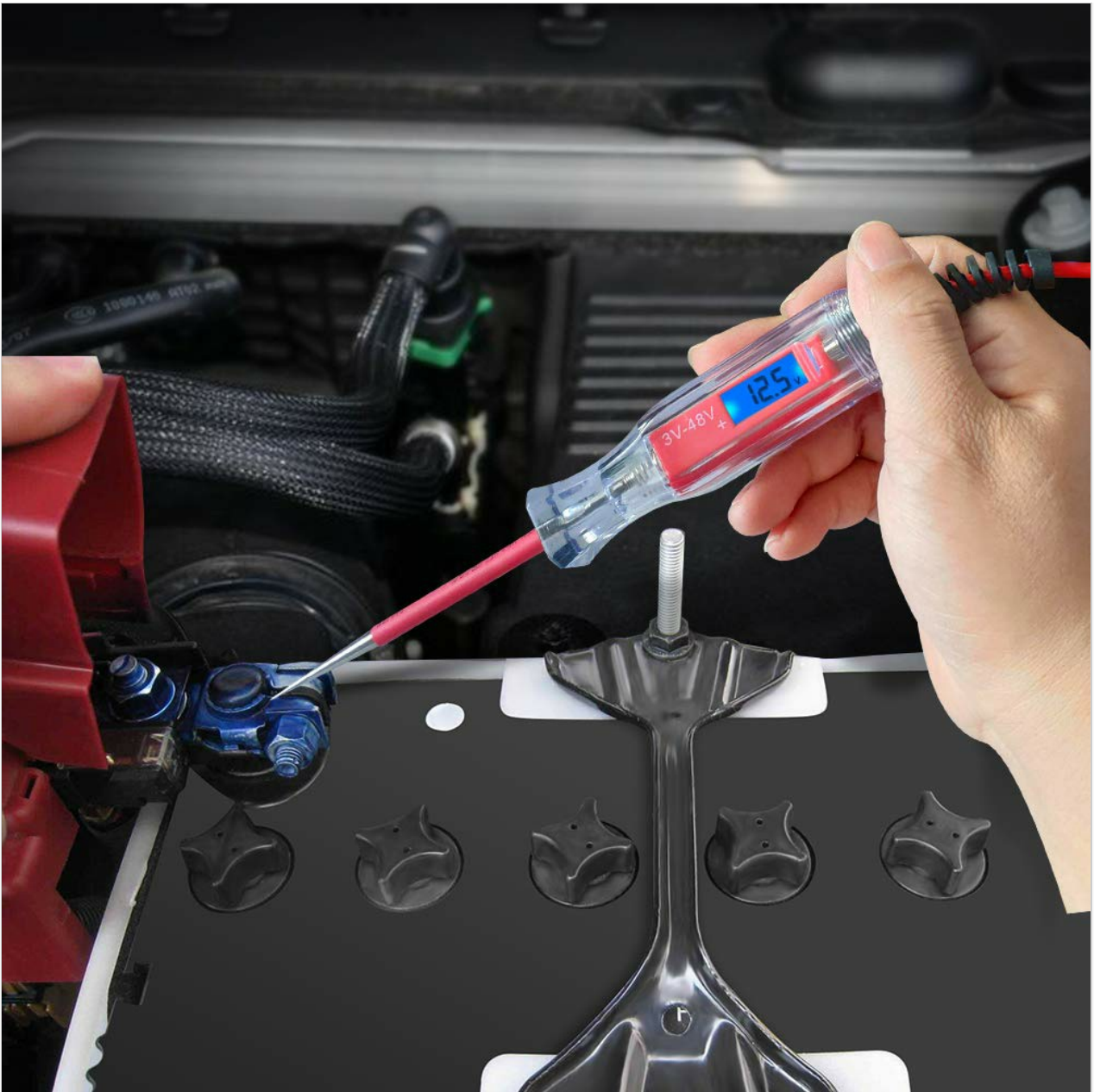
Figure 6: Example of testing a car battery's voltage.
