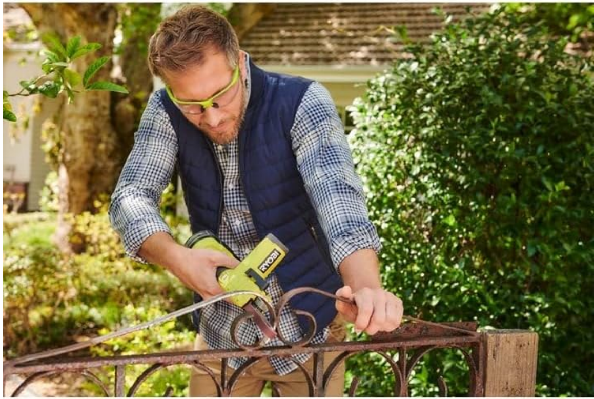
Image 5.2: The tool's narrow belt allows for effective sanding on detailed metalwork, such as an ornate gate.
