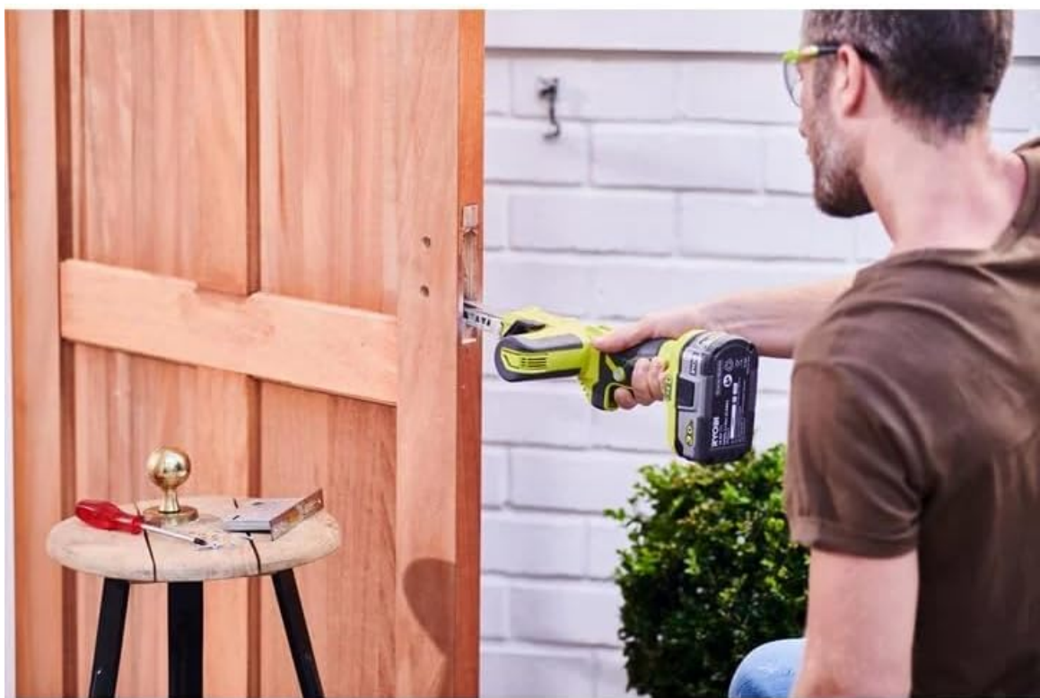
Image 5.3: The power file is used to sand a door frame, highlighting its utility for finishing tasks.
