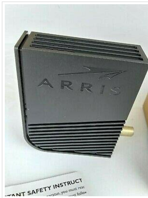
Figure 3: Side view of the Arris MEB1100 MoCA to Ethernet Bridge. This image shows the device from a slightly elevated side angle, emphasizing its compact form factor and the ventilation grilles on the top surface. The coaxial connector is visible at the bottom right.
