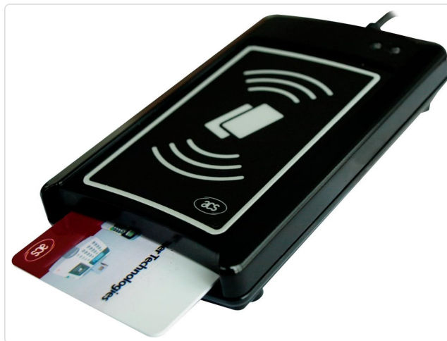
Figure 2: The ACR1281U-C1 reader demonstrating a contact smart card inserted into its designated slot.
