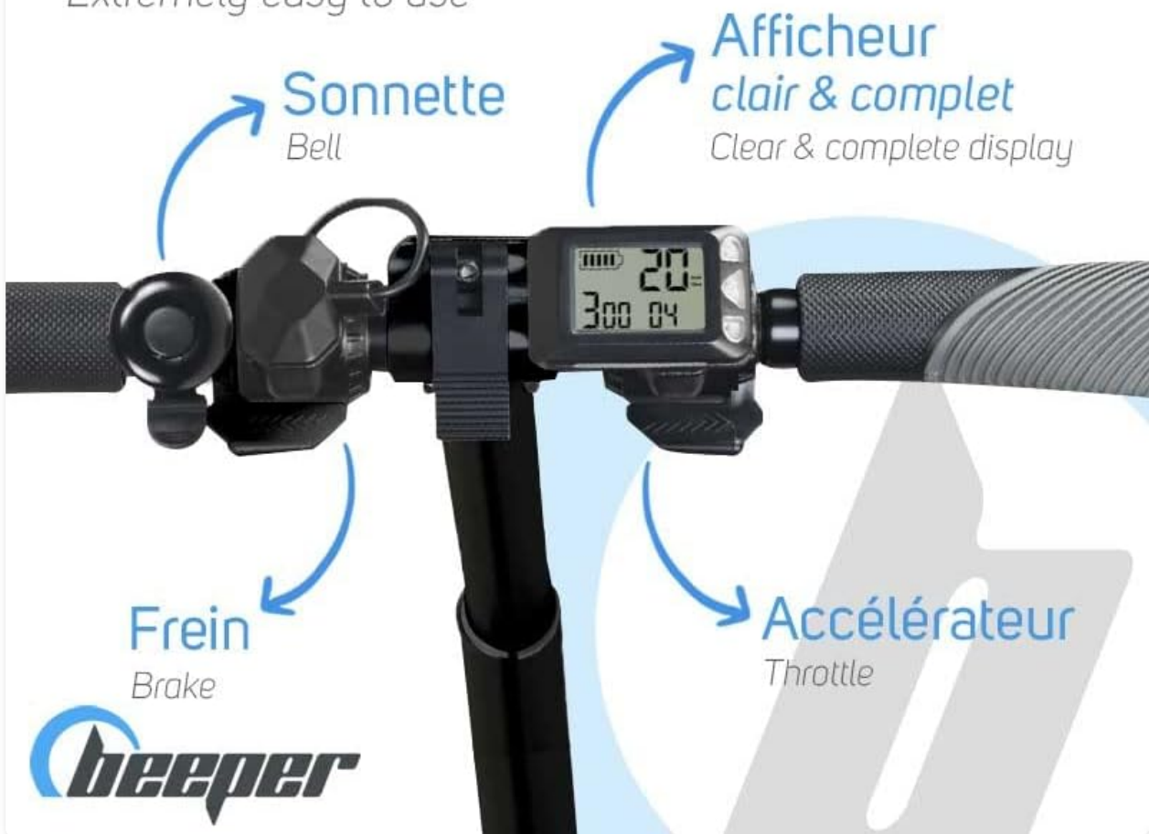
Figure 3.1: Handlebar controls including bell, brake, display, and accelerator.
