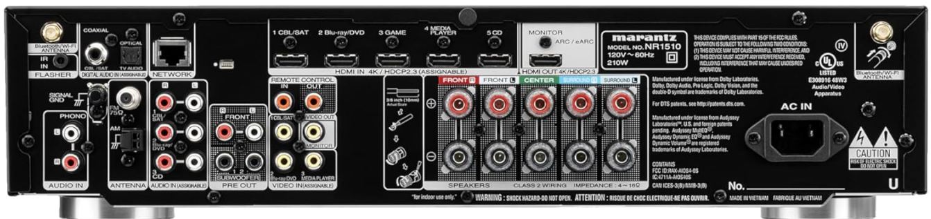
Rear panel of the Marantz NR1510, displaying various input and output ports including HDMI, optical, coaxial, and speaker terminals.
