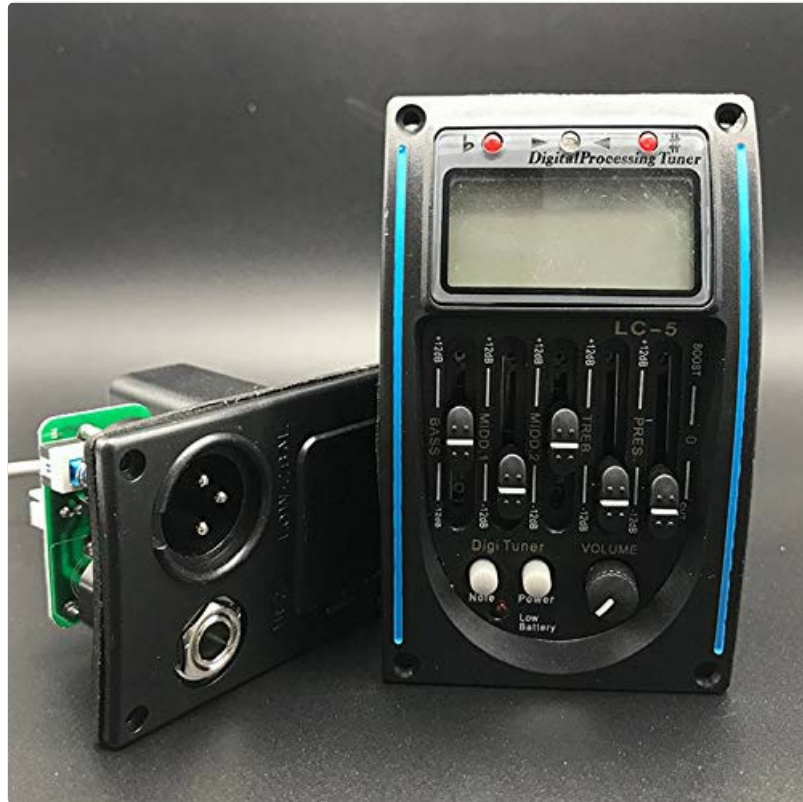
Figure 3.2: Side view of the LC-5 preamp unit, illustrating the output jacks (XLR and 1/4-inch) and the integrated battery compartment.
