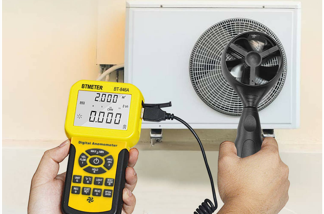
Figure 5: Measuring wind velocity and temperature with the anemometer.
