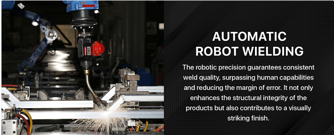
Image 4.1: Depiction of the automatic robotic welding process used in manufacturing, ensuring precise and strong weld seams for the hitch's structural integrity.
