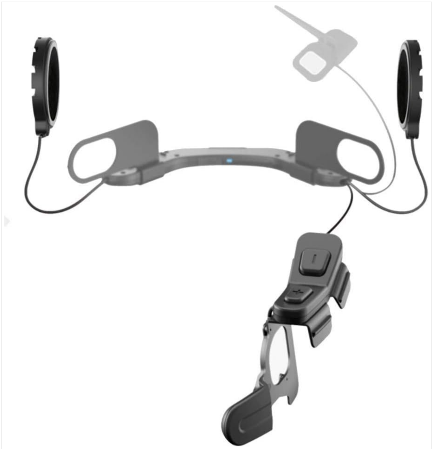
Image: Diagram showing the intended placement of the SC10UA main unit within the helmet's neck roll and speakers in the ear recesses.
