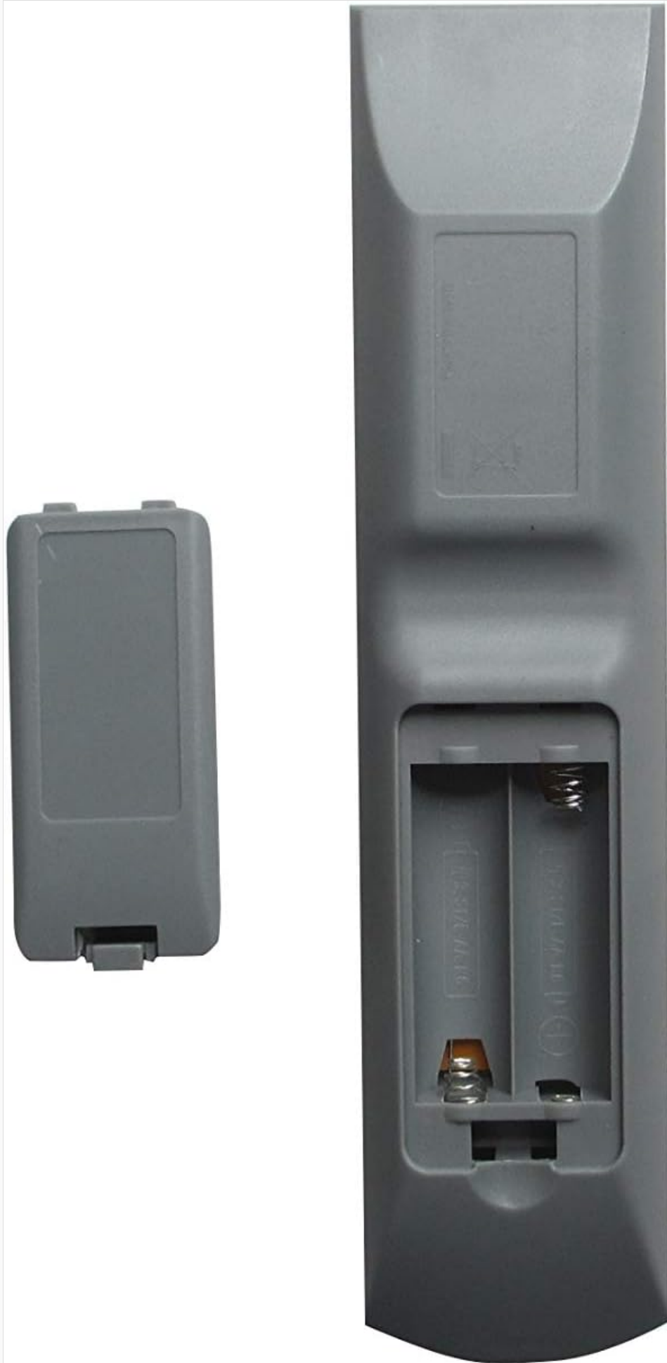
Image: Rear view of the remote control with the battery cover detached, illustrating the battery compartment where two AA batteries are to be inserted. Note the polarity markings.
