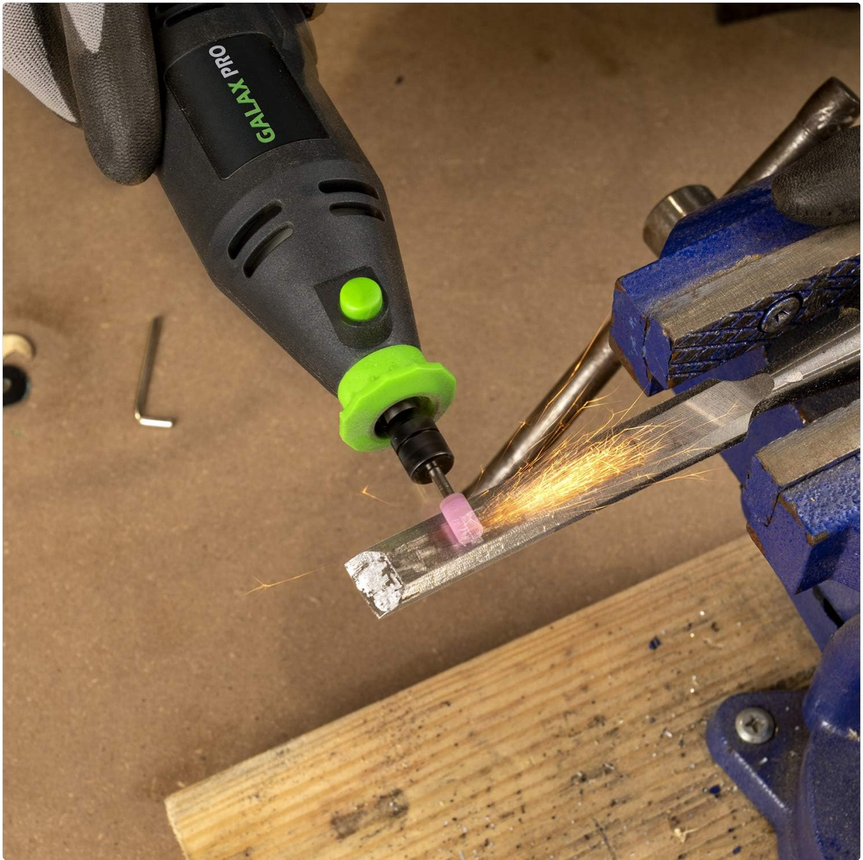
Image: The rotary tool being used to grind a metal chisel, illustrating its capability for sharpening and material removal on hard surfaces.
