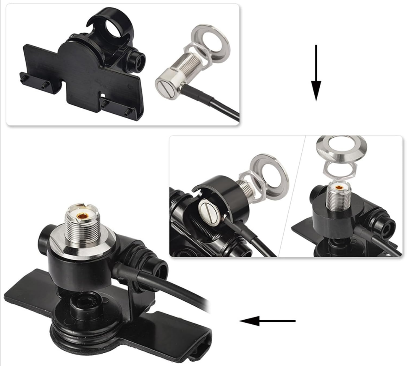
Image: Step-by-step visual guide for assembling the lip mount bracket and attaching the antenna base. The image shows the bracket components, the SO239 female connector, and the final assembled mount.
