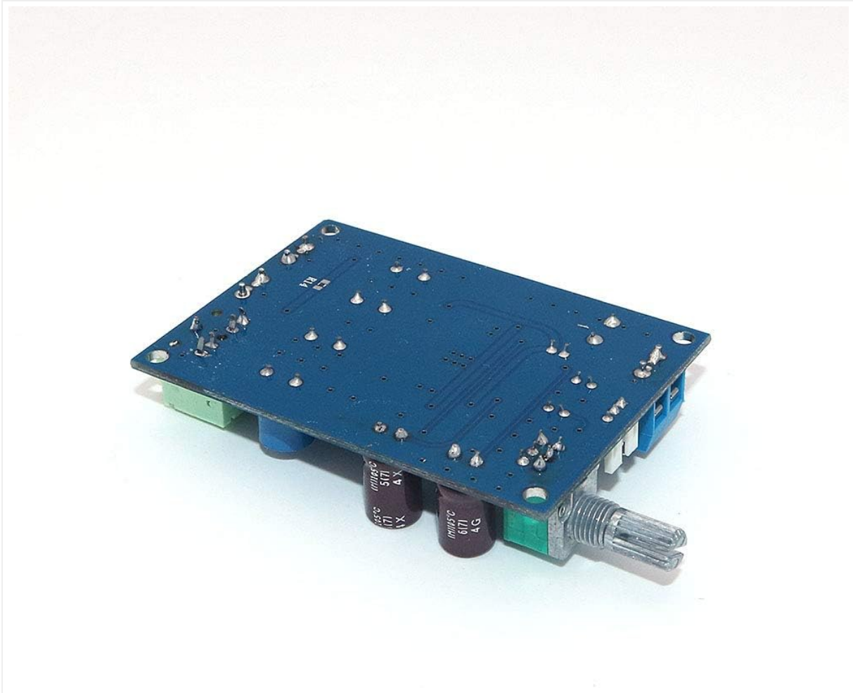
Figure 4: Bottom view of the amplifier board, illustrating the solder points and circuit traces. Proper handling is essential to prevent damage to these components.
