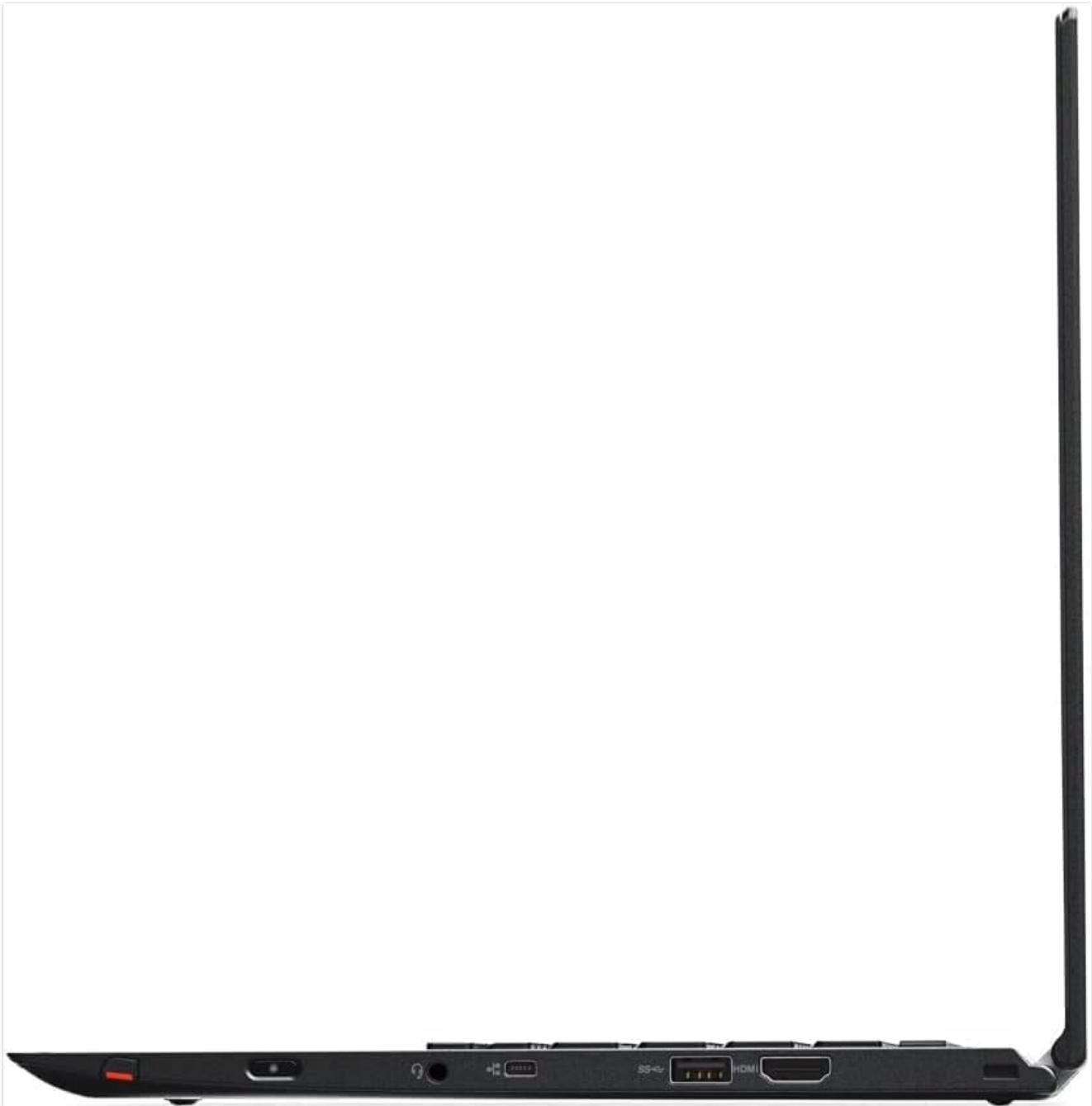
Image: Left side of the laptop, illustrating port locations for power and peripherals.
