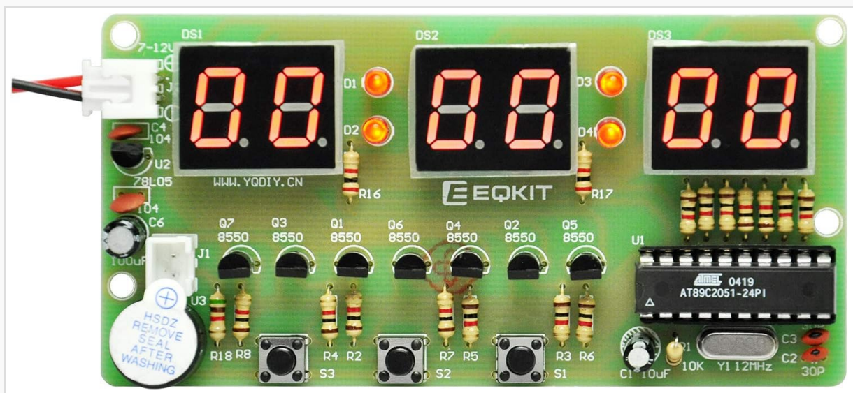
Image 5.1: The assembled clock module, highlighting the three control buttons on the PCB.
