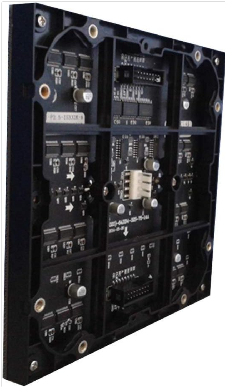
Image 2: Side-rear perspective of the LED matrix panel, providing a clearer view of the module's depth and the arrangement of its electronic components and connectors.
