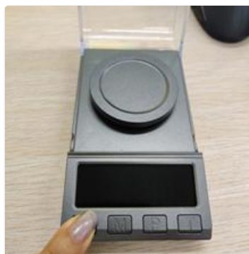
Image: Changing weighing units using the 'M' button.
