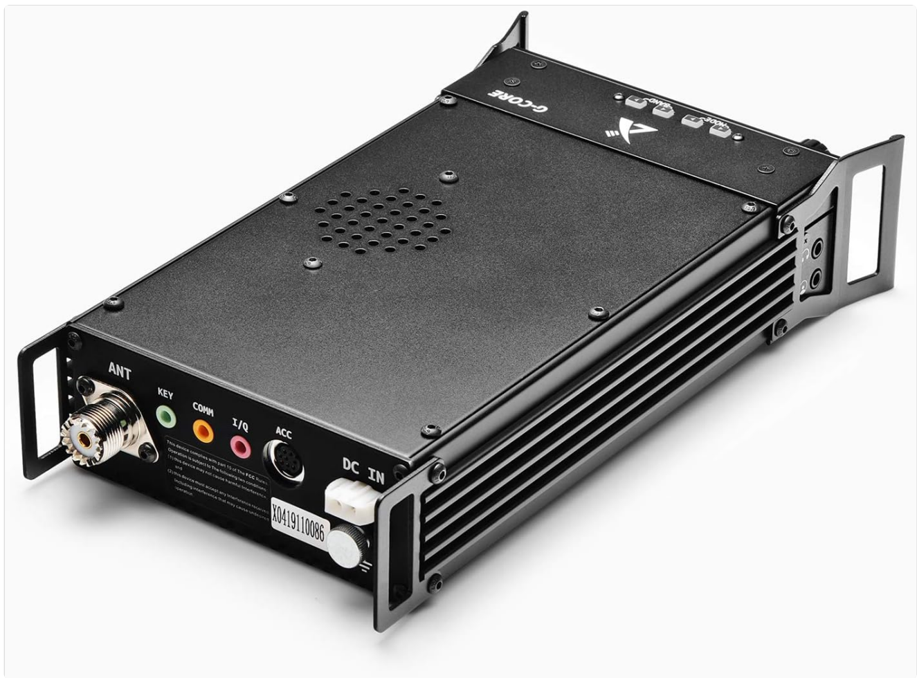
Image: The rear panel of the Xiegu G90, displaying various connection ports including ANT (antenna), KEY, CONN, I/Q, ACC, and DC IN.
