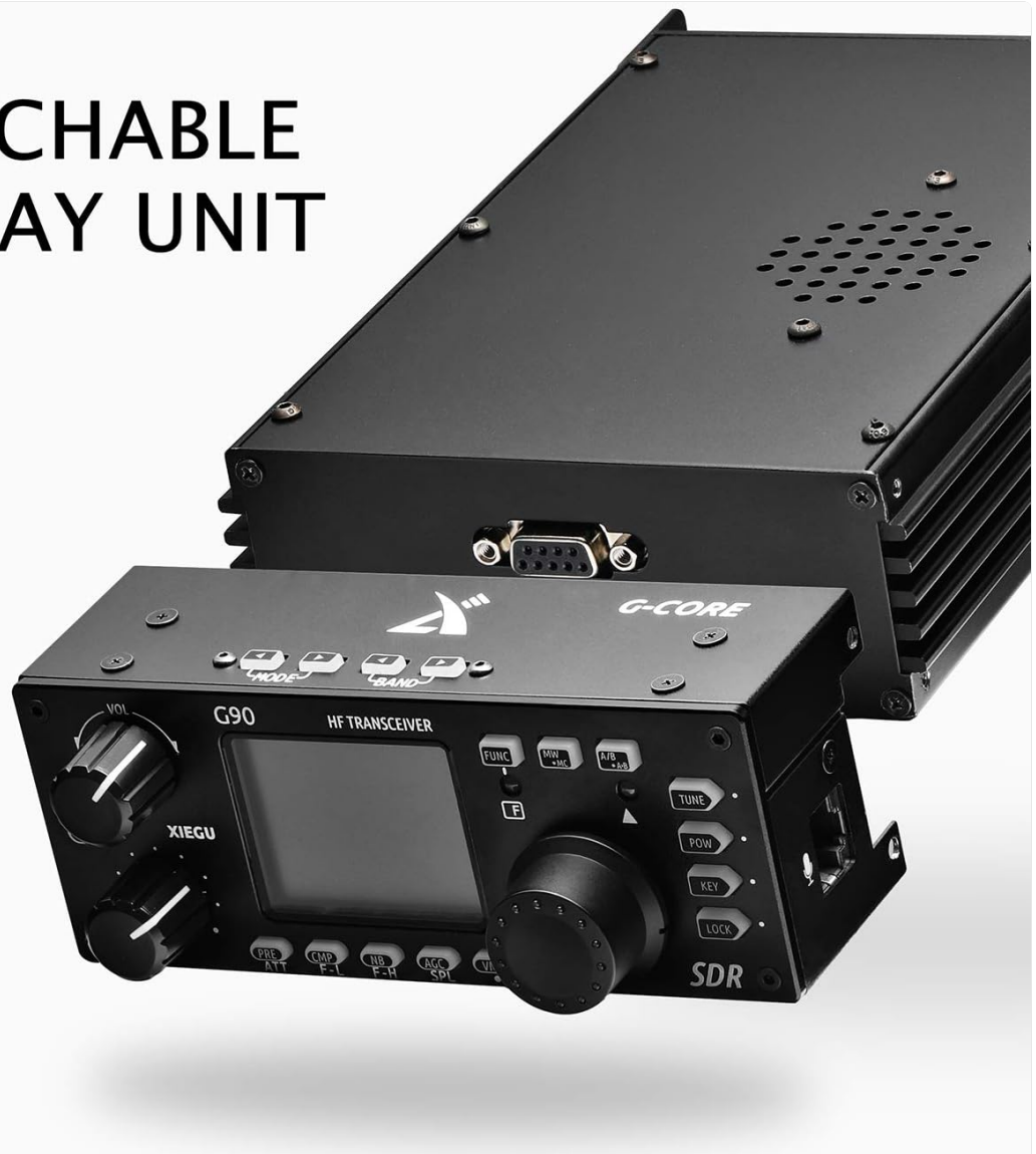
Image: The Xiegu G90 with its display unit detached from the main body, illustrating the modular design.
