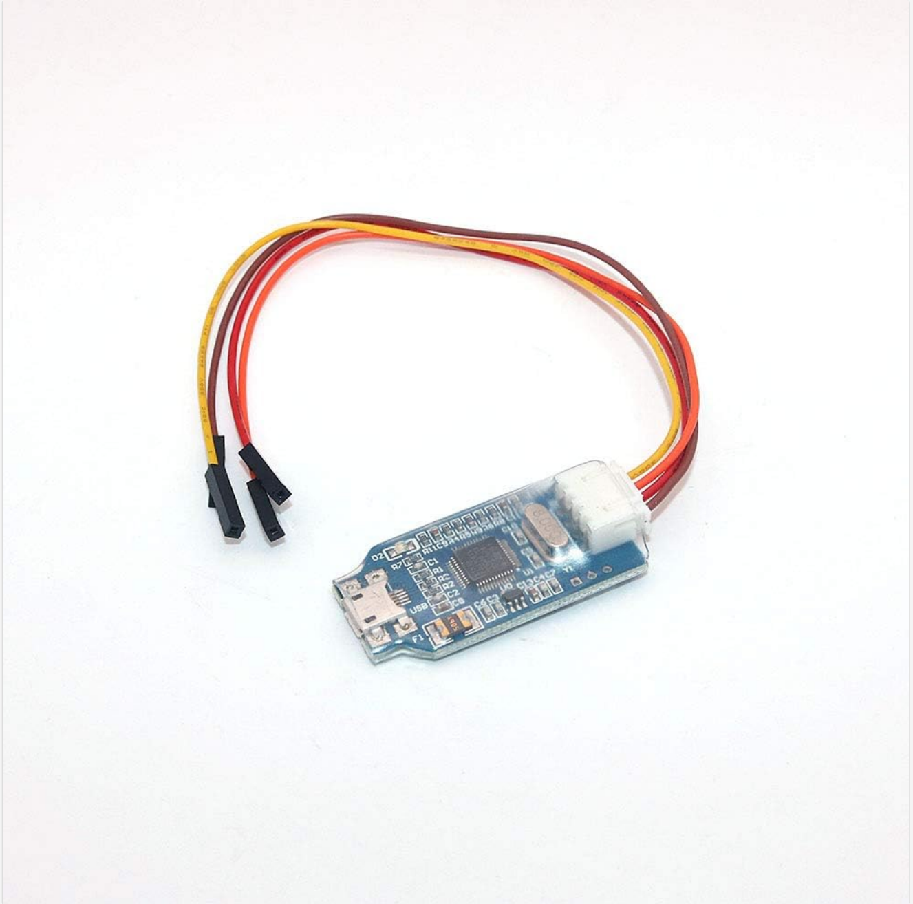
Figure 3.2.1: Top view of the DolaTek T86 Link with connected wires, showing the microUSB port and pin headers.
