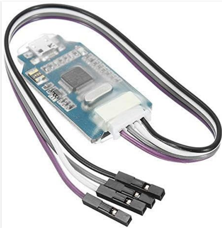
Figure 4.2.1: The DollaTek T86 Link with various colored jumper wires, indicating its readiness for connection to a target device.
