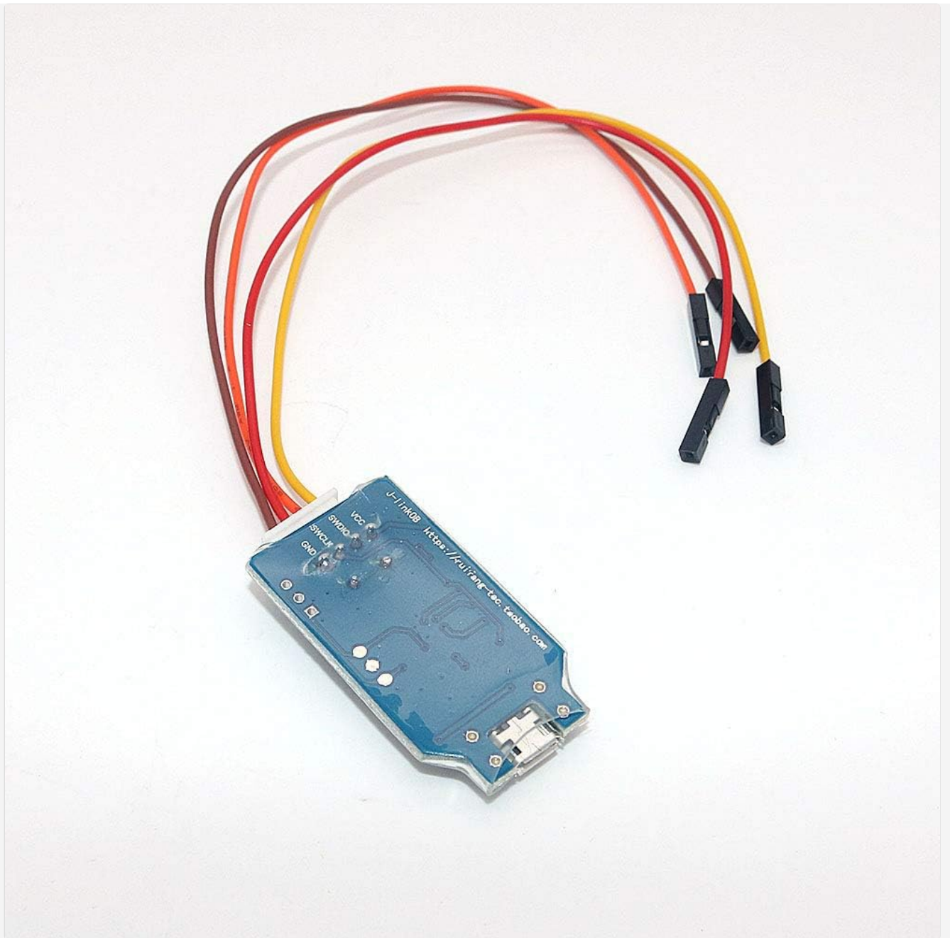
Figure 3.2.2: Bottom view of the DollaTek T86 Link, clearly labeling the SWDIO, SWCLK, and GND pins for connection.
