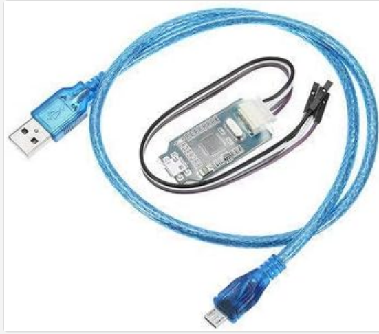
Figure 3.3.1: The DollaTek T86 Link connected to a blue USB cable, illustrating a typical setup for PC connection.
