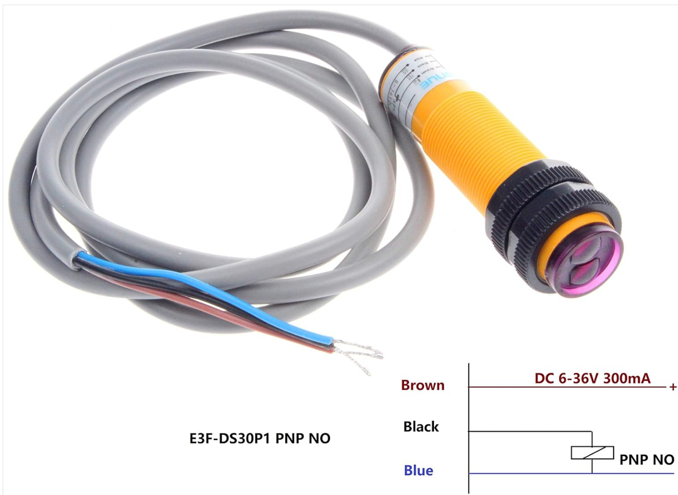
Figure 3.1: Wiring diagram for the E3F-DS30P1 PNP NO sensor. The brown wire connects to DC 6-36V positive, the blue wire to negative, and the black wire is the PNP NO output.
