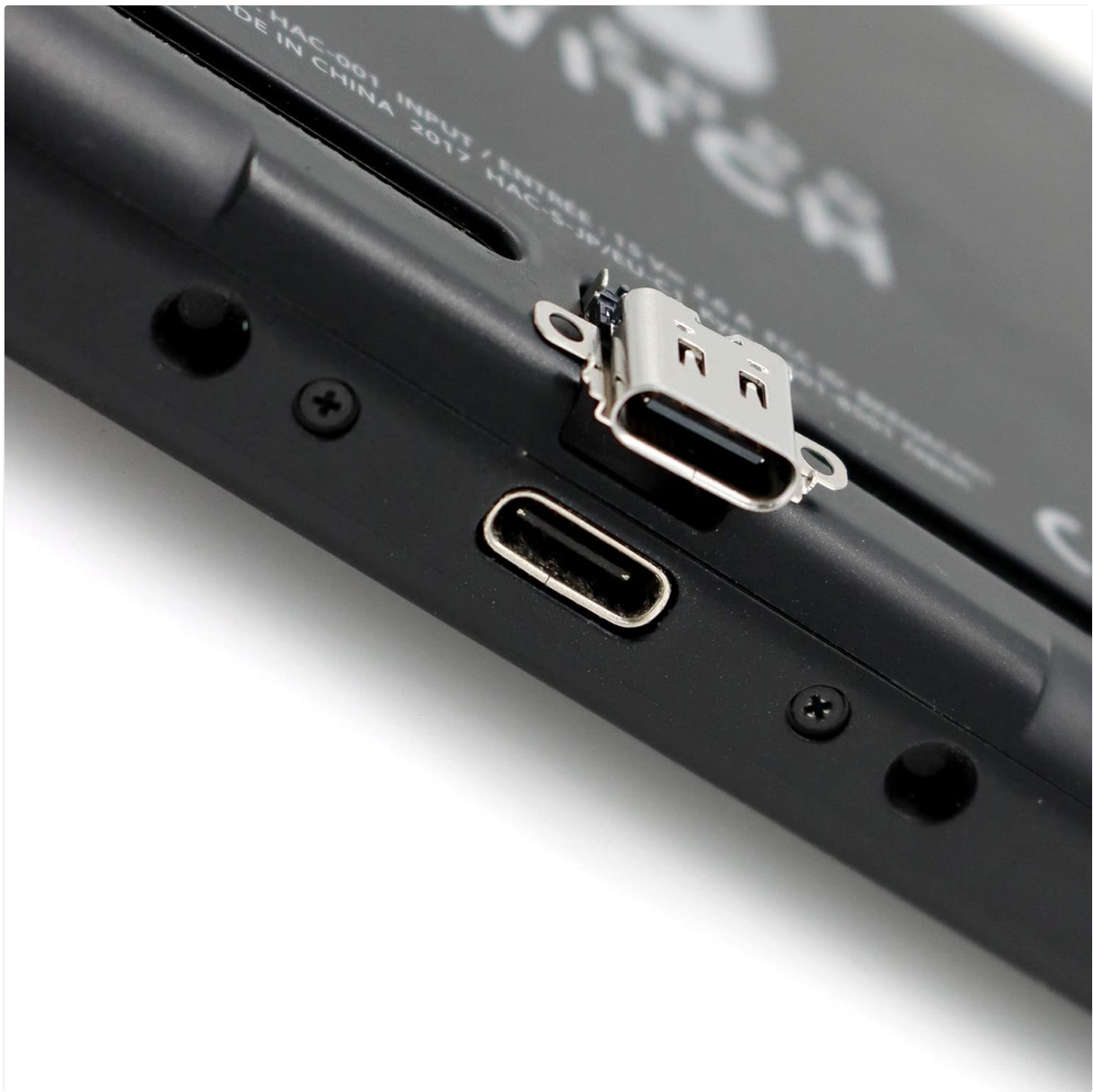
Image 4.1: The replacement USB-C port positioned next to a Nintendo Switch console, illustrating its intended location.
