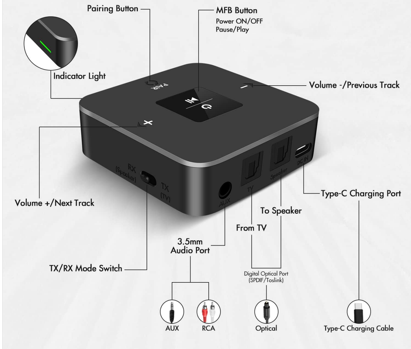
Figure 4: Detailed view of the Giveet BTI-038, labeling its buttons, indicator light, mode switch, and various audio ports (AUX, Optical, Type-C charging).
