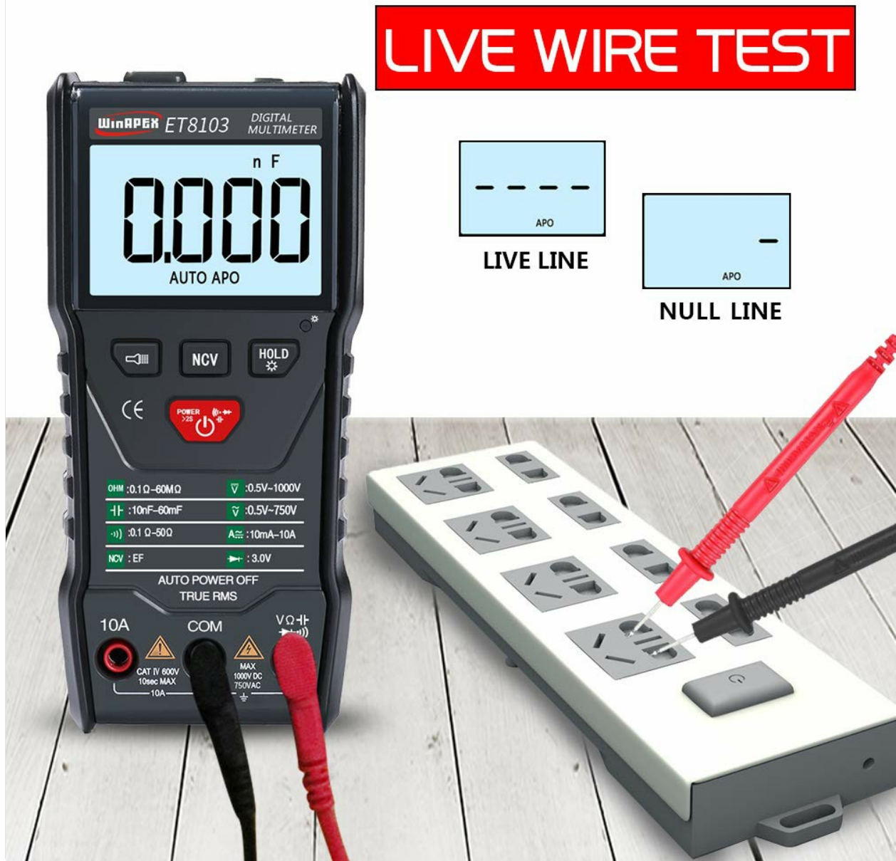
Figure 6.2: Performing a live wire test.
