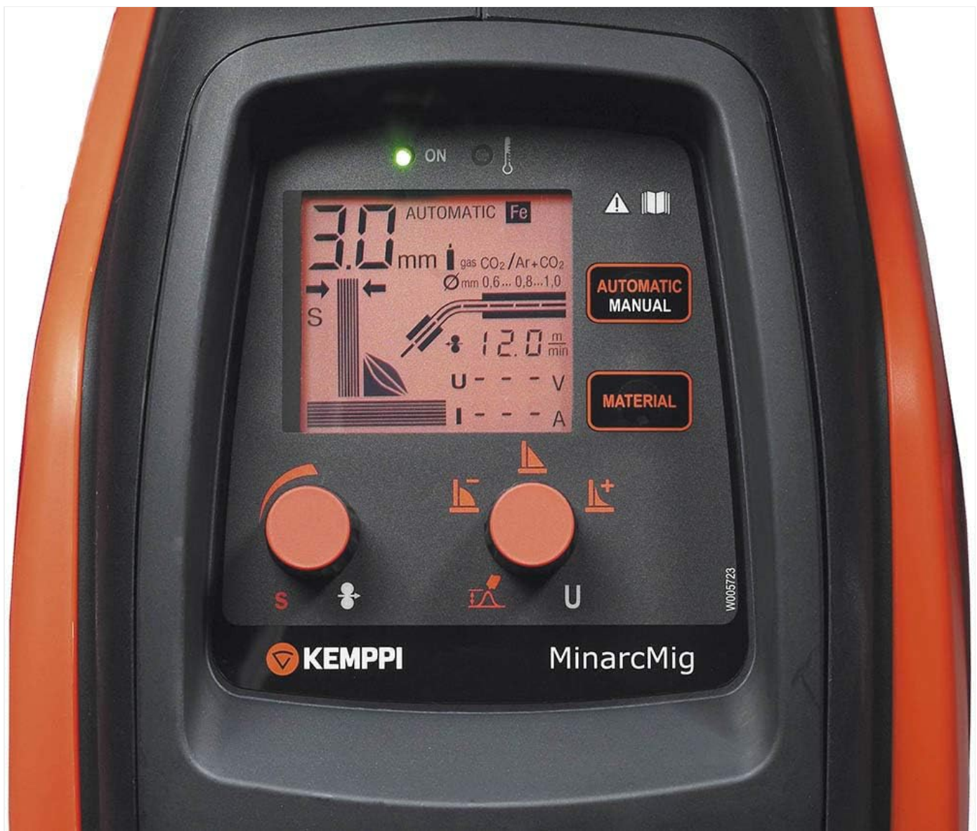
Figure 3.3: Close-up of the control panel, displaying the digital screen, adjustment knobs, and mode selection buttons for automatic and manual operation, material type, and gas settings.
