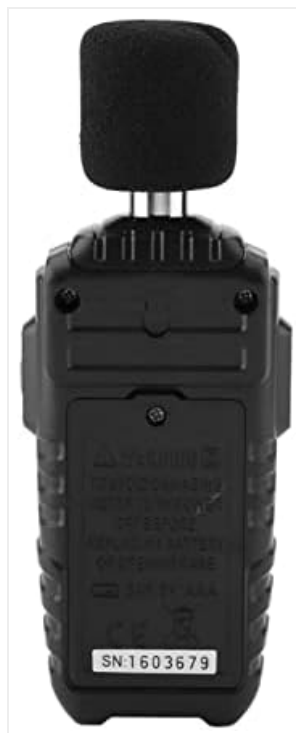
Figure 4.1: Rear view of the sound level meter, showing the battery compartment where three AAA batteries are installed.
