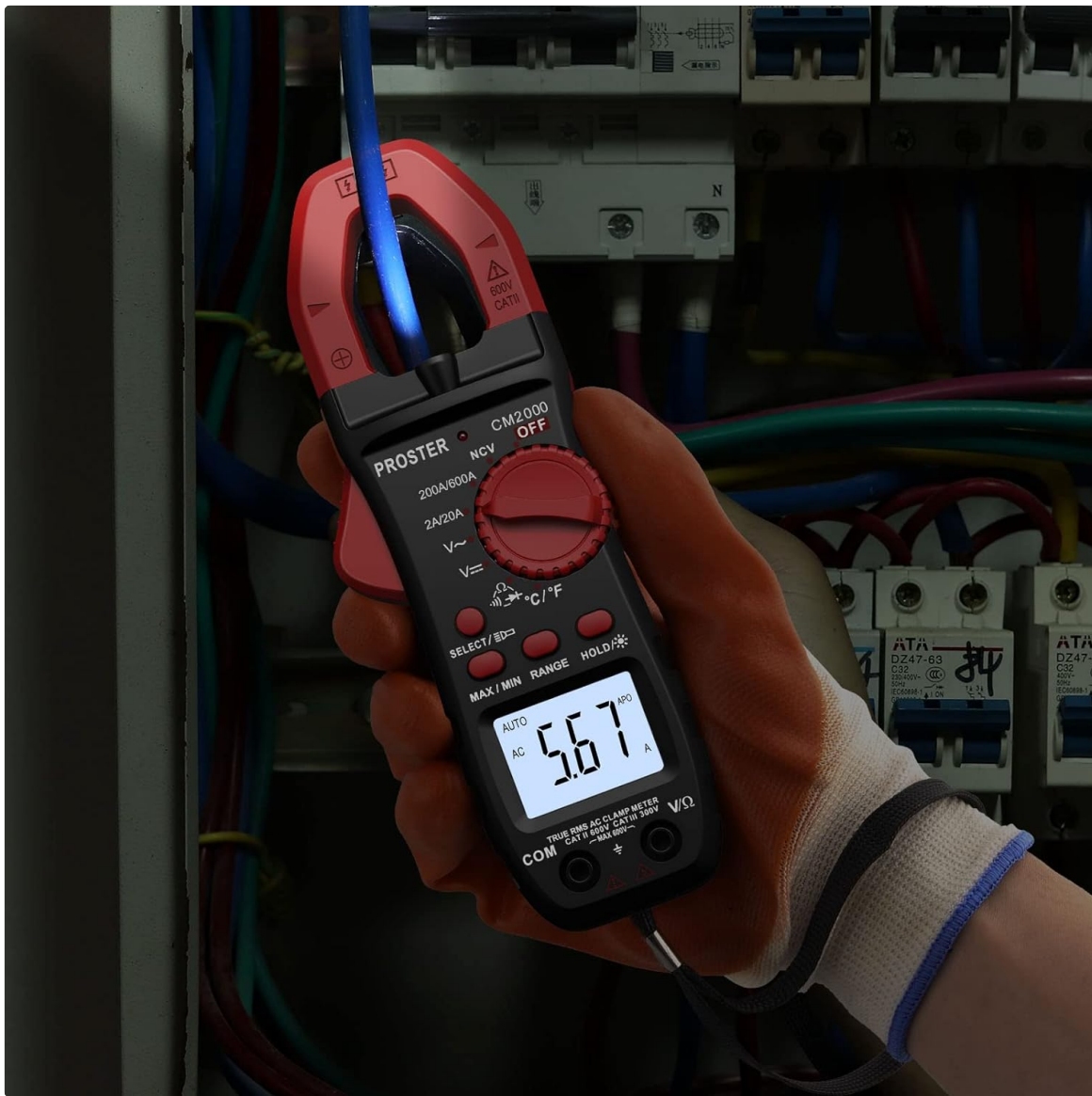
Figure 6.1: Measuring AC current with the clamp jaw.
