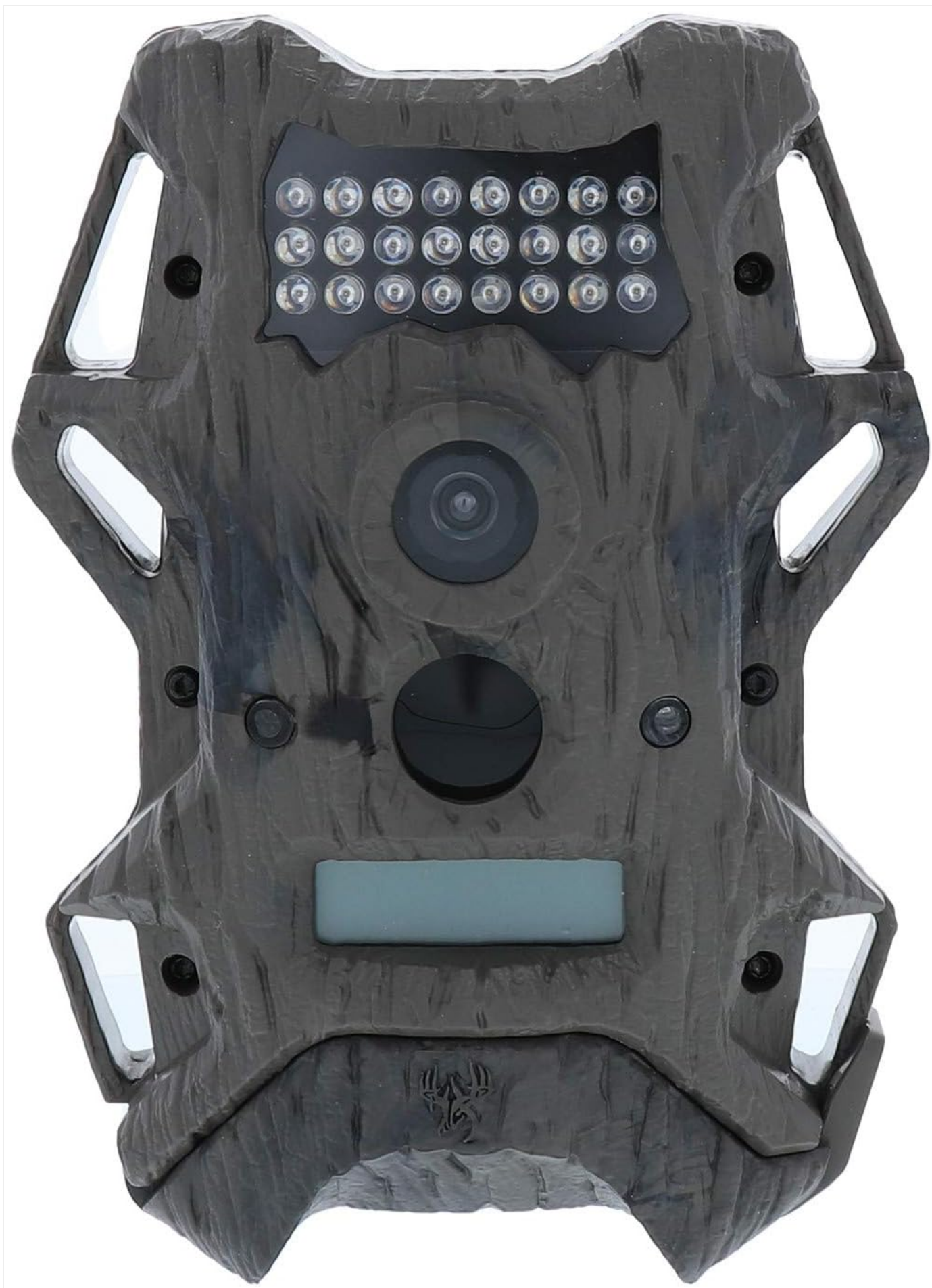
Image 2.1: Front view of the Cloak 14 HD camera, showing the lens, infrared LEDs, and control panel area.
