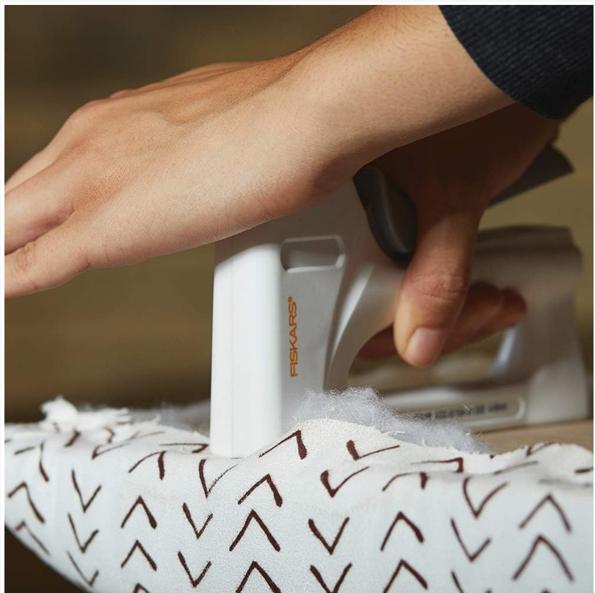
Figure 6.1: A hand demonstrating the use of the Fiskars staple gun to secure fabric. The image shows the staple gun pressed firmly against the material, ready for operation.
