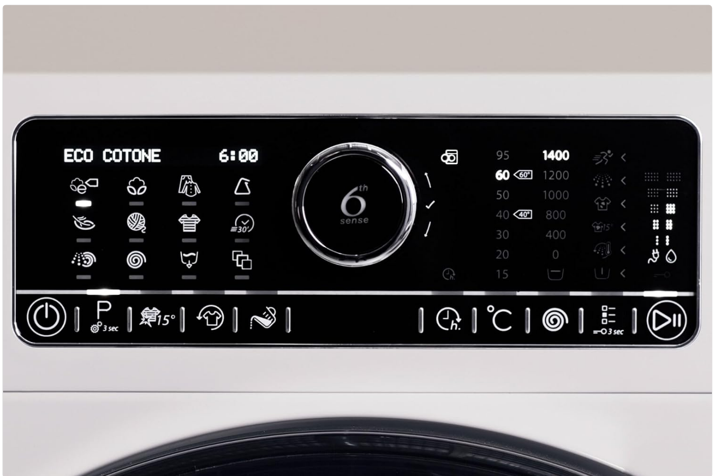
Figure 5: Alternative view of the control panel, showing the central program selector and function buttons.
