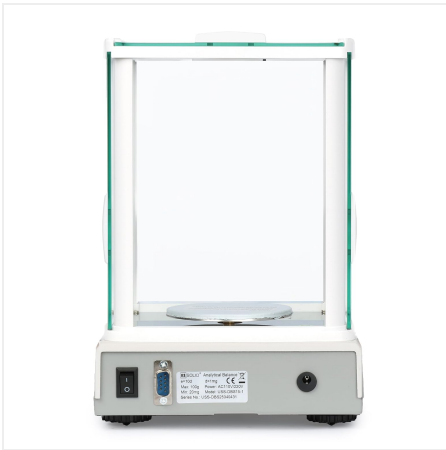
Rear view displaying the power switch and RS232 interface port.
