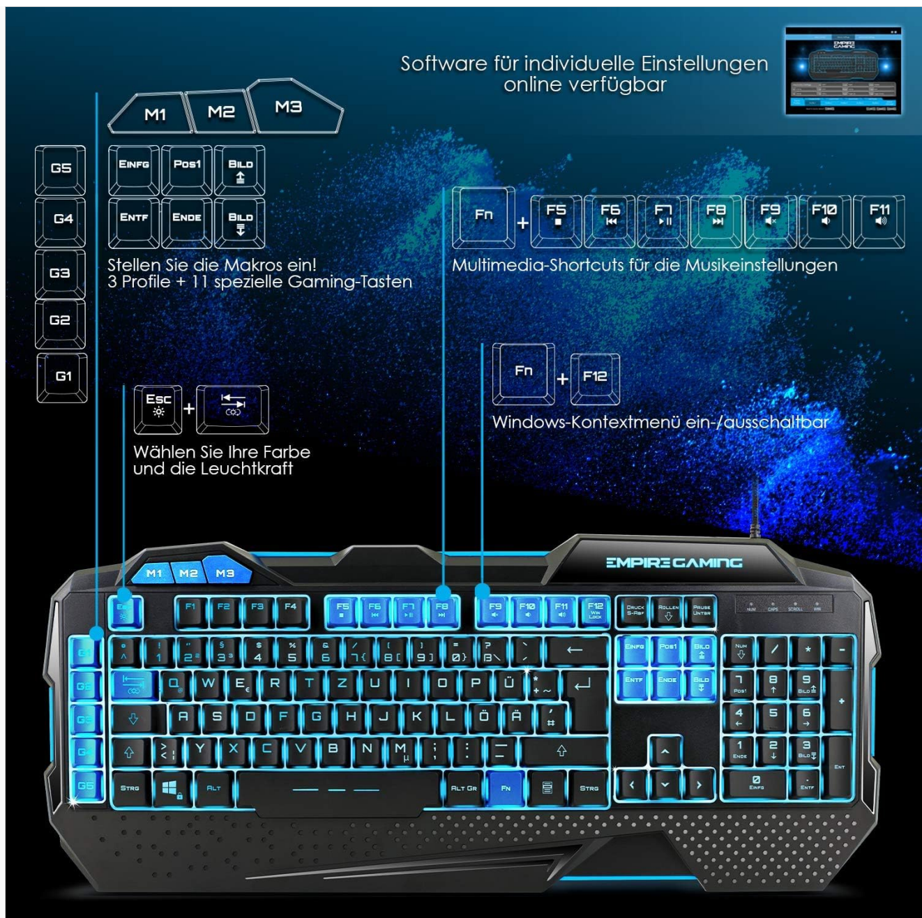
Figure 4: Hellhounds Keyboard layout highlighting macro and multimedia keys.
