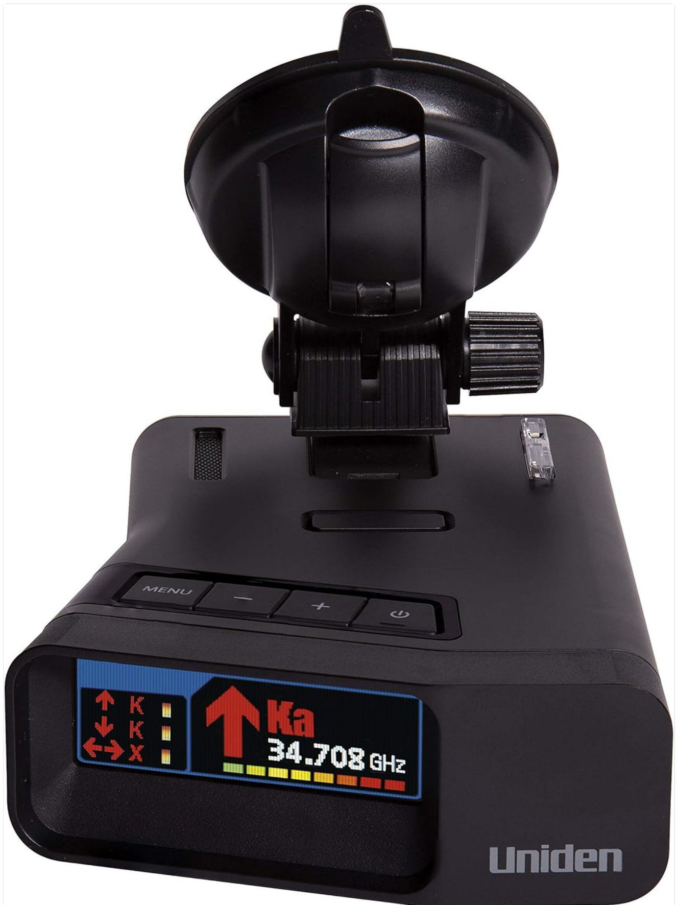
Figure 1: Uniden R7 with single suction cup mount. Ensure a clear line of sight for optimal detection.
