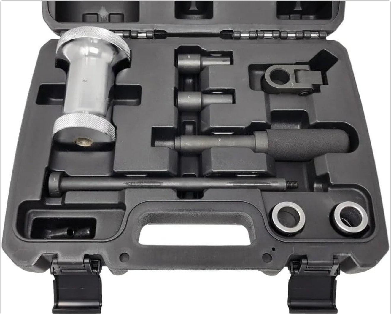
Figure 1: The CTA Tools 7808 Injector Puller Kit neatly organized within its durable storage case.
