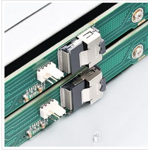
Image: Close-up of the Mini SAS SFF-8087 data connectors on the drive backplane.
