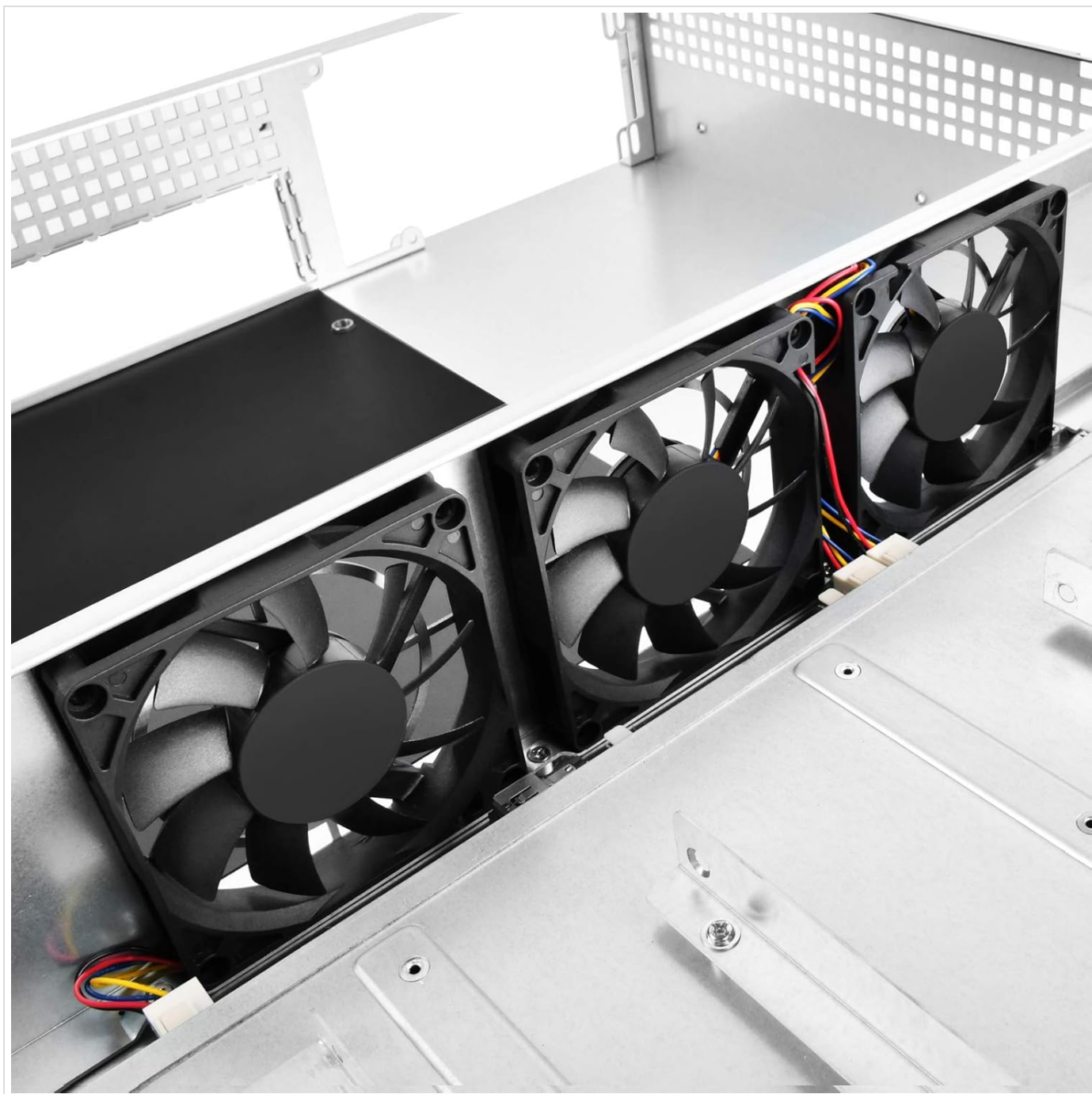
Image: Close-up view of the three 80mm PWM fans mounted internally, responsible for cooling the drive bays and internal components.
