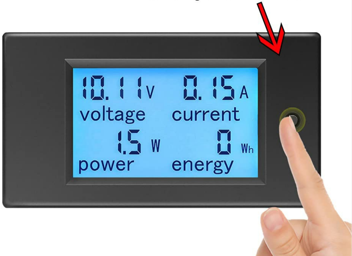
Image: The KETOTEK KT-D138 digital multimeter showing the location of its single control button, used for energy reset, backlight control, and setting the voltage alarm threshold.
