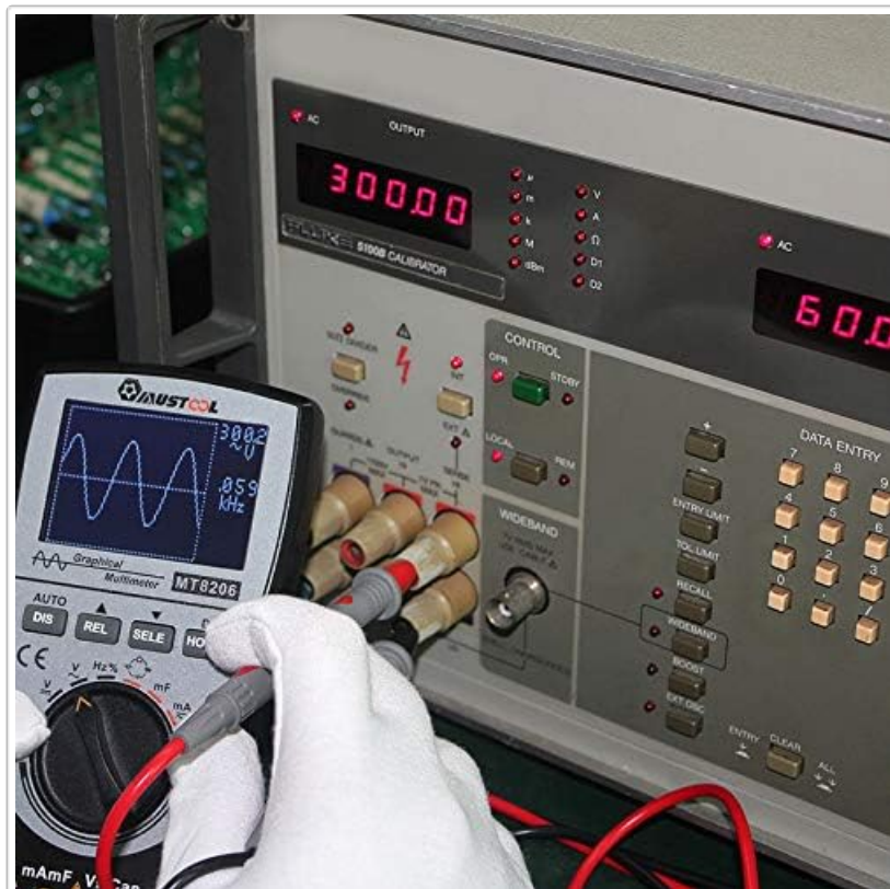
Figure 6.2: MT8206 connected to a calibration device, demonstrating its measurement capabilities.
