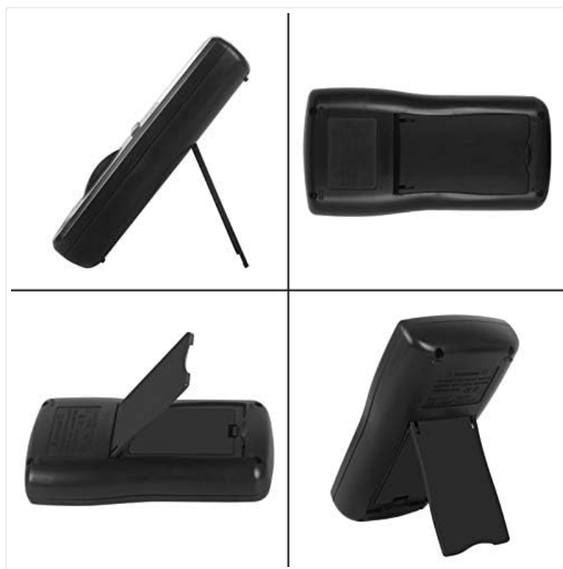
Figure 4.2: Various views of the MT8206, showing the kickstand and battery compartment.
