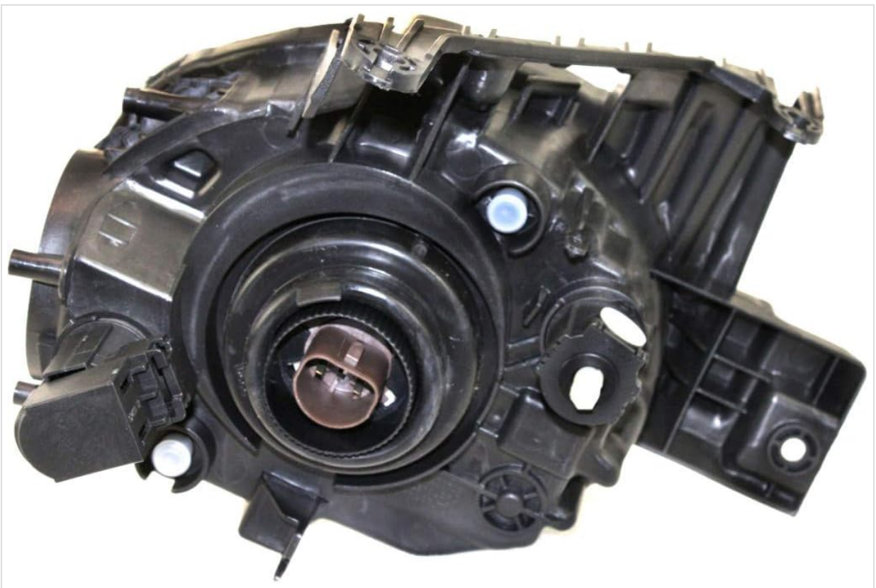
Figure 2: Rear view of the headlight assembly, illustrating the bulb access points and electrical connectors.
