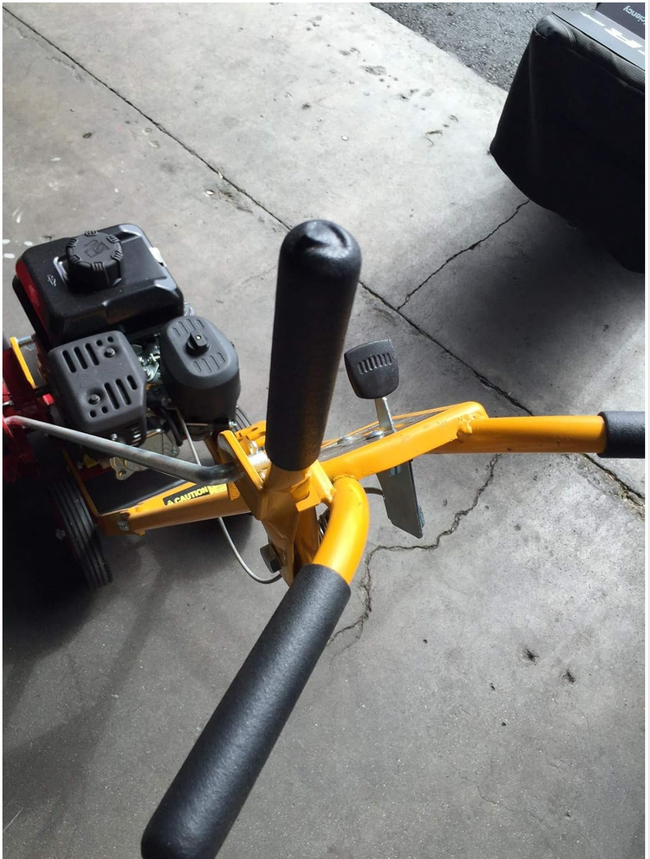
Figure 6: Top view of a McLane machine's handlebar, showing a typical mounting area for the throttle control.
