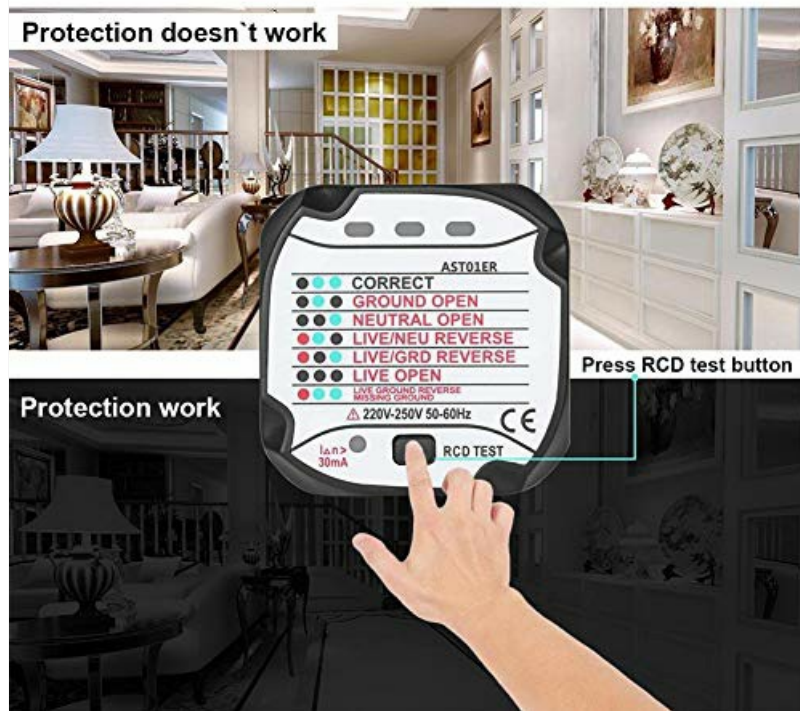
Image 5.2: Performing an RCD test by pressing the dedicated button.
