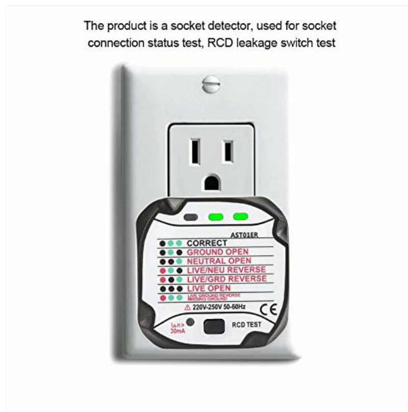
Image 5.1: The socket tester plugged into an outlet, indicating correct wiring.
