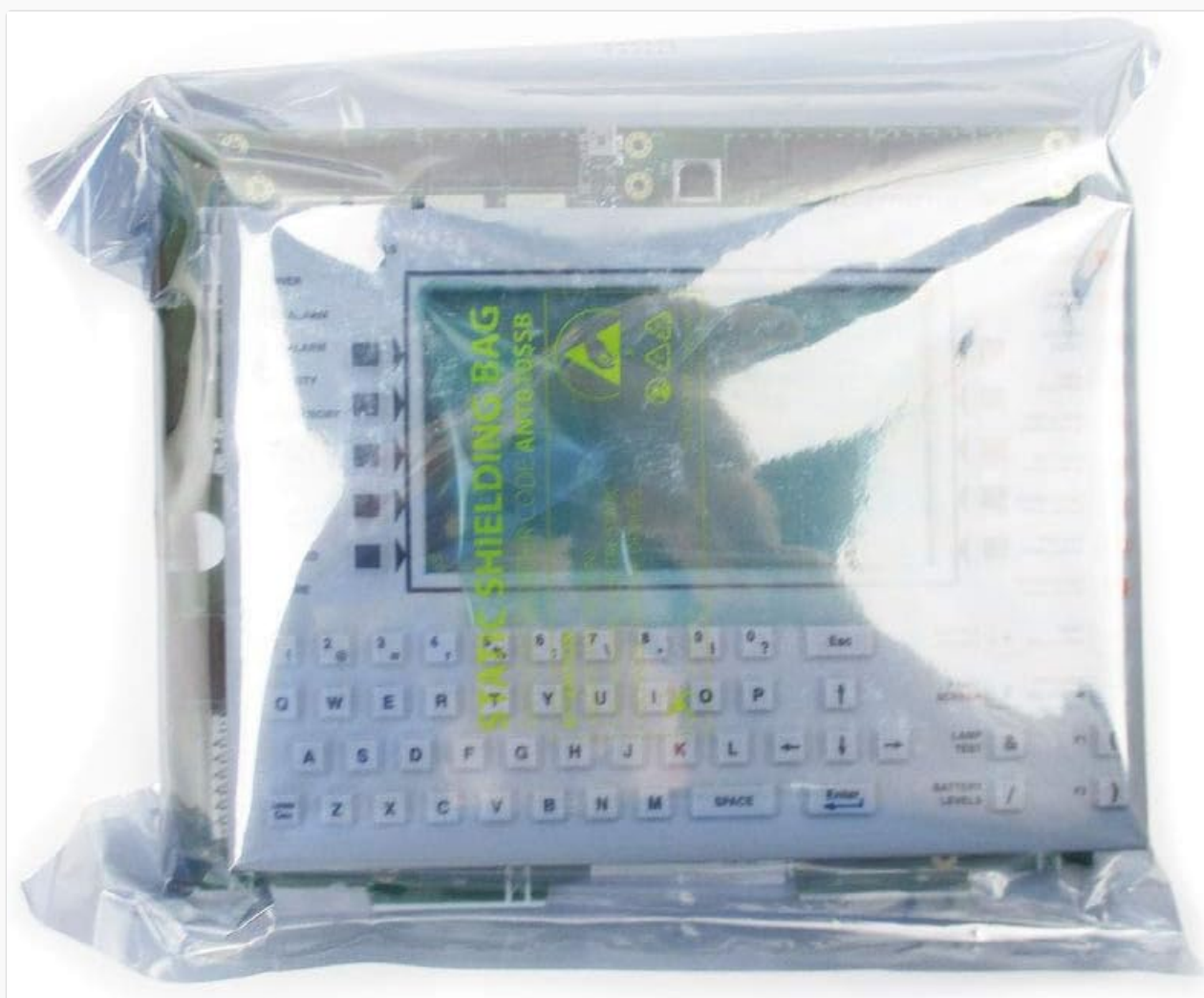
Figure 2.2: The Notifier NCA-2 unit, protected within an anti-static shielding bag, showing its display and keypad through the
