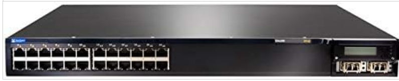
Figure 4.1: Front Panel of EX4200-24P Switch. This image displays the front of the Juniper Networks EX4200-24P switch, featuring 24 RJ-45 Gigabit Ethernet ports, each with LED indicators, and four SFP+ uplink ports on the right side, along with a small LCD display and control buttons.
