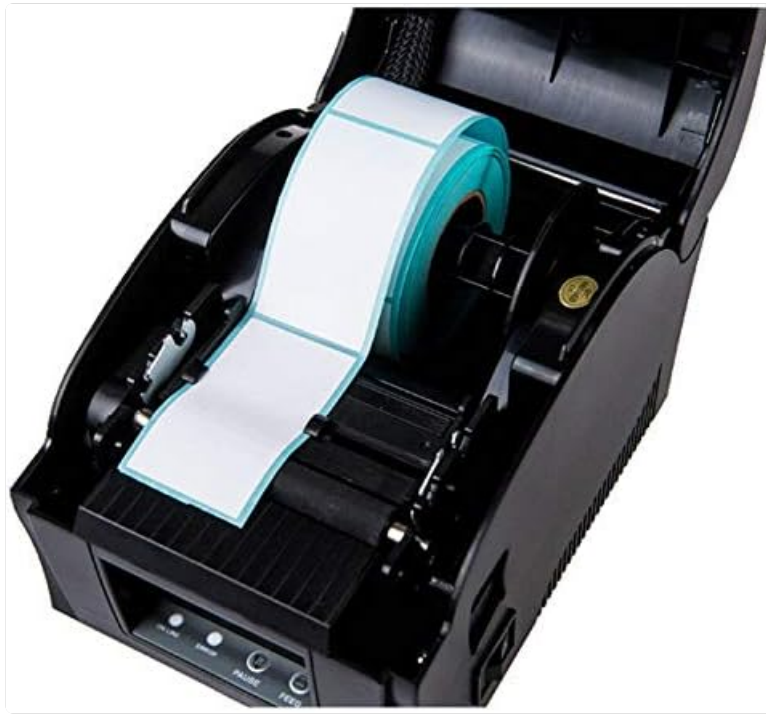
Figure 5.1: Loading a roll of thermal labels into the XP-360B printer's internal compartment.
