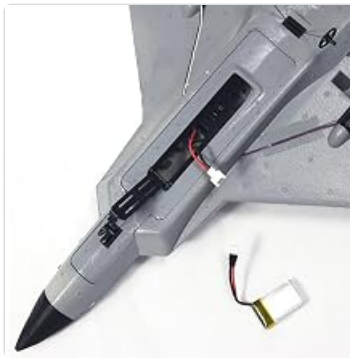
Image: A close-up view demonstrating the correct method for inserting the battery into the aircraft's battery compartment.
