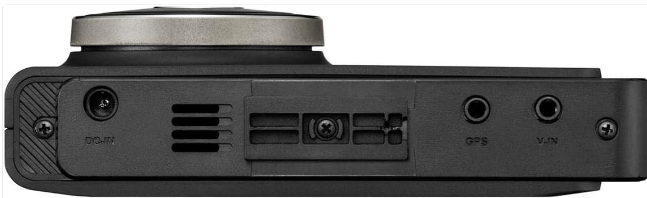
Image 3.3: Side view of the X700 main unit, displaying the DC-IN power input, GPS antenna port, and V-IN port for the rear camera connection.
