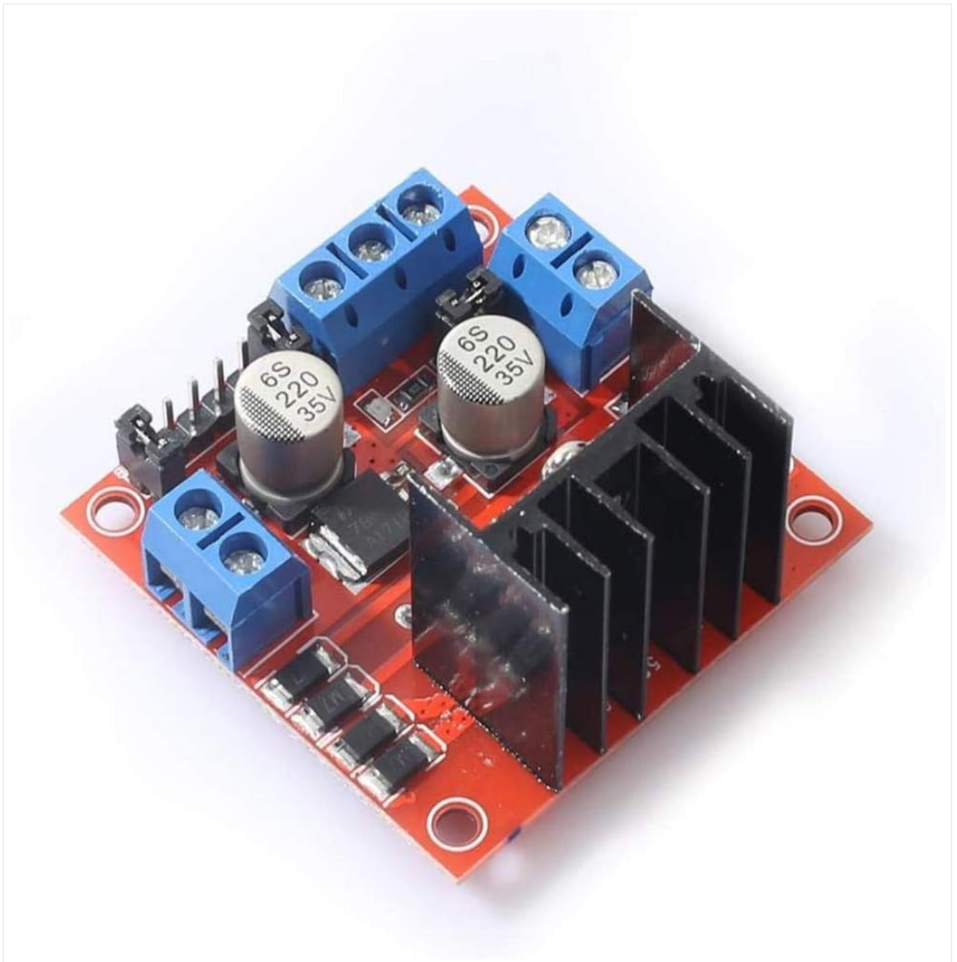
Figure 3: Angled view of the L298N module, highlighting the input/output terminals and heatsink.
