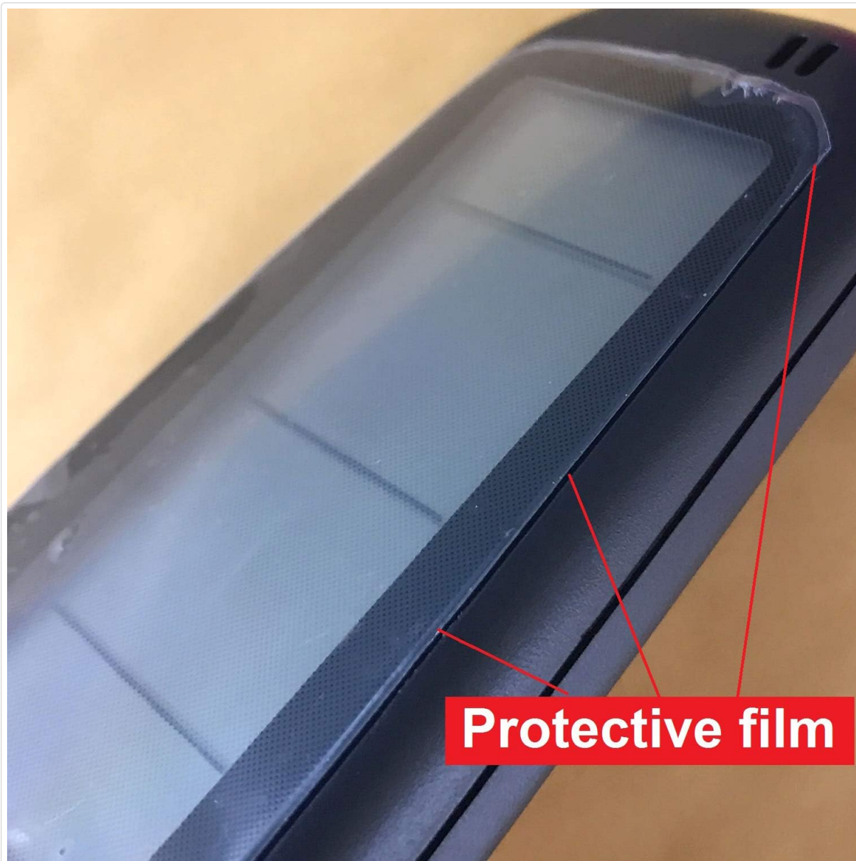
Figure 2: Protective Film. Before first use, gently peel off any protective film from the remote control's LCD screen to ensure clear visibility.
