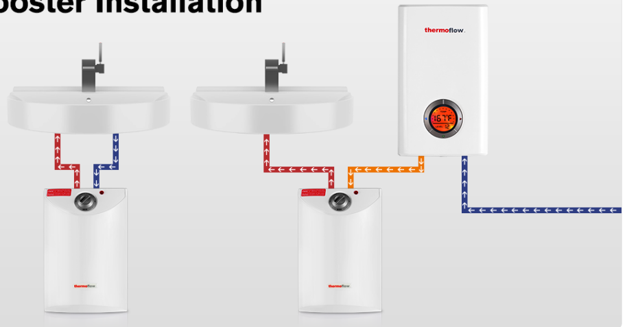
Image: Diagram illustrating two installation methods: connecting the mini tank water heater directly to a single faucet, and connecting it in series with an existing water heater to boost hot water.
