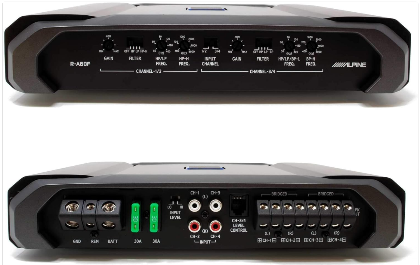
Figure 2: Control panel (top) and input/output terminals (bottom) of the Alpine R-A60F amplifier.
