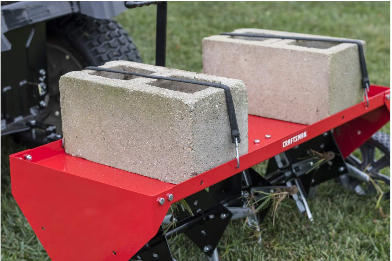
Image: A close-up shot of concrete blocks resting on the aerator's weight tray, secured with straps.
